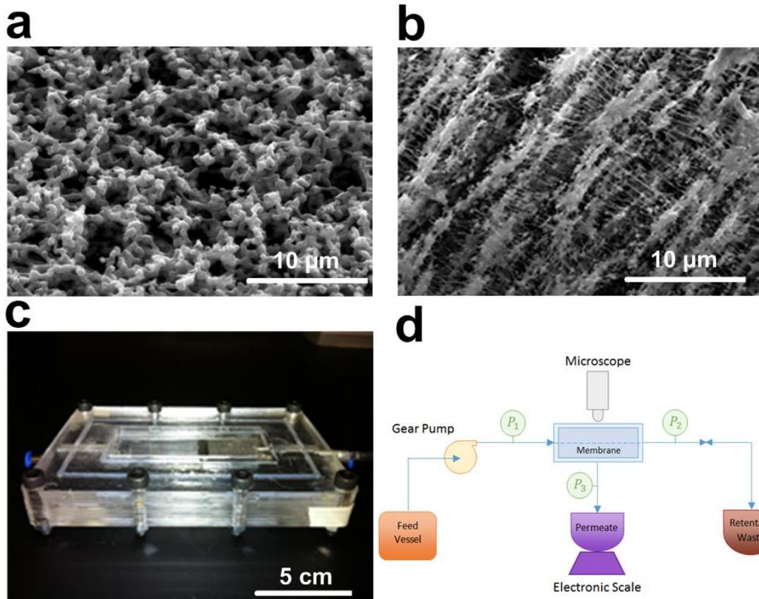
**Figure S5.** (a) & (b) SEM photos of the Cellulose (Millipore, Cat. No. AAWP04700) and Teflon filter (Pall, Cat. No. P5PL047) with nominal pore size of around  $1 \mu\text{m}$  used in this study for yeast separation. (c) Optical image of the cross-flow filtration setup made from PMMA and used for microfiltration tests. (d) Schematic representation of the experimental setup used for the tests.
