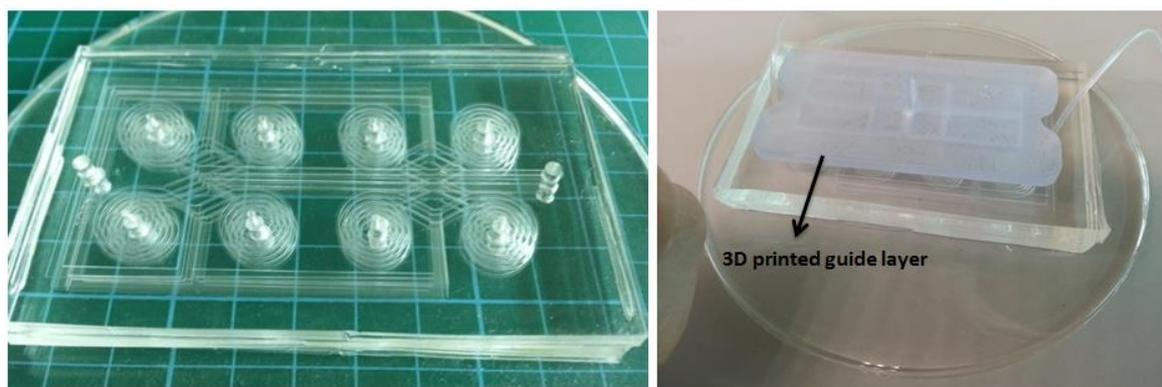
**Figure S3.** Optical image of a multiplexed inertial microfiltration system designed for separation of yeast cells. Similar to our system developed for mammalian cell retention, this system also consists of multiple layers of PDMS sheets with embossed microchannels bonded together for continuous cell retention from large sample volumes. The microchannels used in this system has also trapezoidal cross-section with  $30 \times 70 \mu\text{m}$  channel dimensions.
