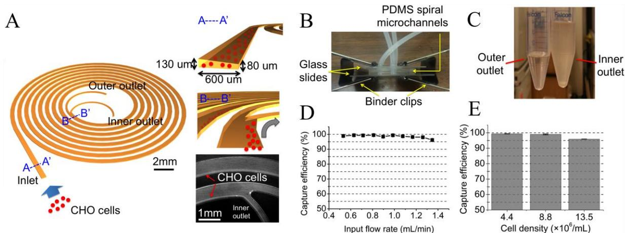
Figure 1: (A) The schematic of the spiral microfluidic channel. Most cells were focused into the inner wall in the spiral channel whereas cell-free solution was collected in the outer outlet. (B) The glass-PDMS-glass sandwich spiral microchip for robust operation. (C) Sample solution from spiral channel outlets. (D) Capture efficiencies according to different input flow rates. Two devices were used. (E) Capture efficiency dependence on input cell density.
